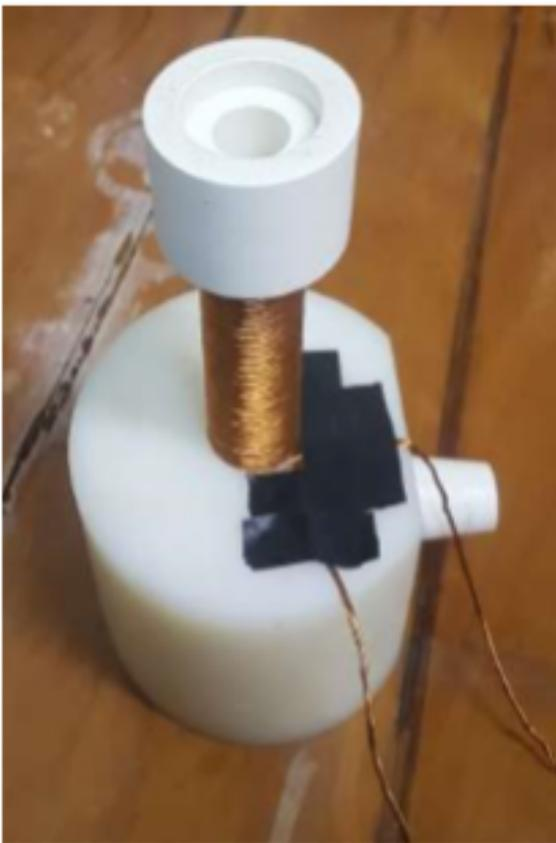
Figura 2.6: Bobina principal enrolada com fio de Litz.
